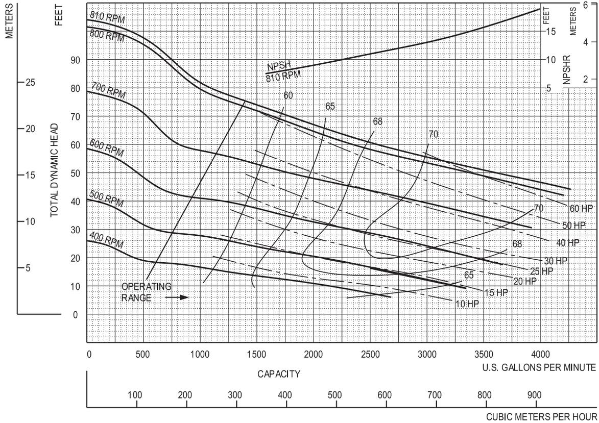
Performances shown are for cool water, close-coupled electric configuration with Cyclo Seal.® Other mounting configurations, seal arrangements or liquids may require horsepower and/or performance adjustments.
