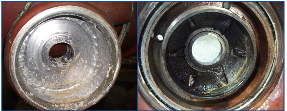
ON LEFT: Volute shows signs of severe wear.
