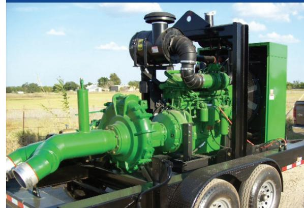
DOUBLE SUCTION SET UP ALLOWS FOR MAXIMUM FLOW TO THE PUMP, BUT ALSO MAKES FOR EASIER HANDLING VS. A 12" LINE WHICH WOULD BE REQUIRED FOR THE SAME FLOWS IN A SINGLE LINE.
