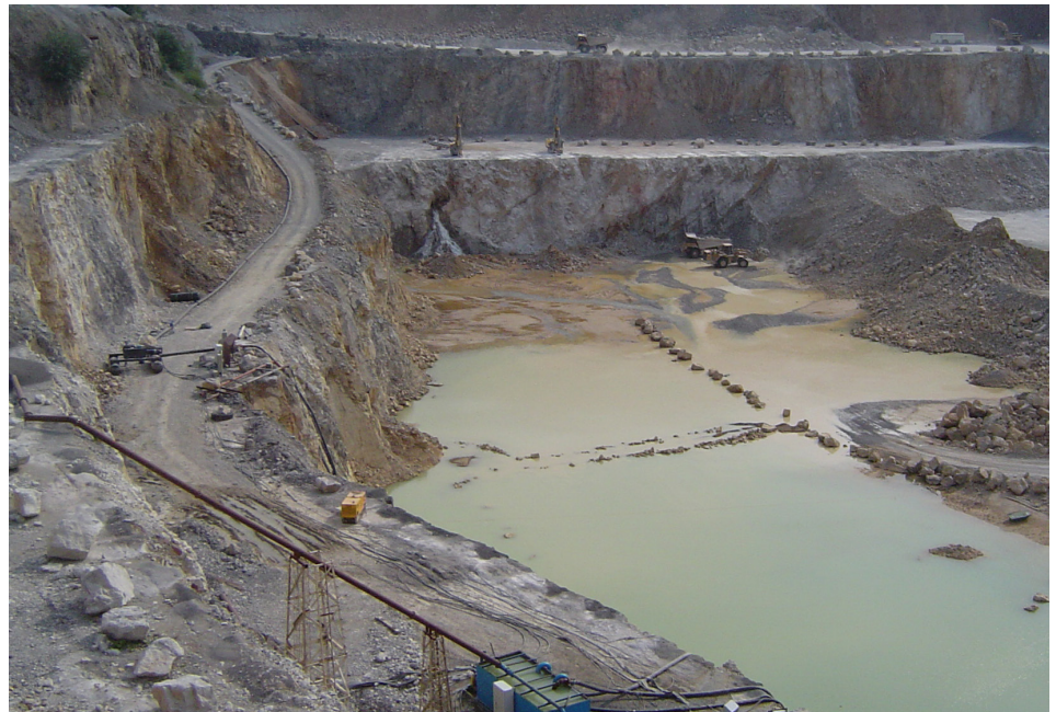
Mining sites like the quarry shown above can benefit from remote monitoring for pumps that are running while the operation is unmanned during dewatering.
